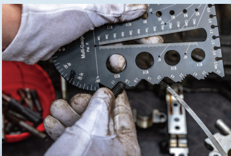
Pitch Size : Measure the Thread
