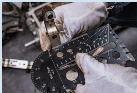
Bolt Length : Measure Length
