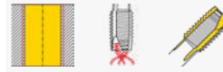
through holes up to 2,5 x D Chip removal (like picture) Form B with spiral point
